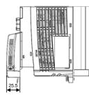
After mounting option adapter, the depth of inverter is 25.5mm up.
