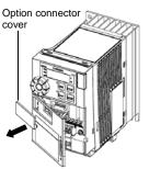
2 Remove the option connector cover on control terminal cover
